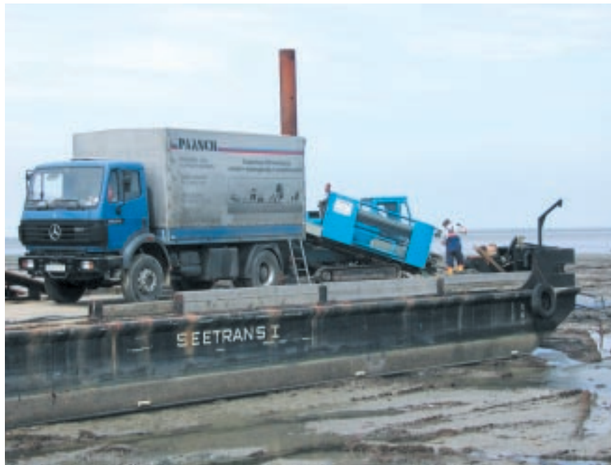
The pontoon carrying the boring equipment.
